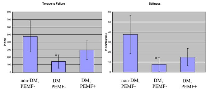
Figure 2. Mechanical Testing. The data represents averages ± SD. \* Represents values statistically lower than non-DM, and DM+ PEMF values,  $P<0.05$ .
